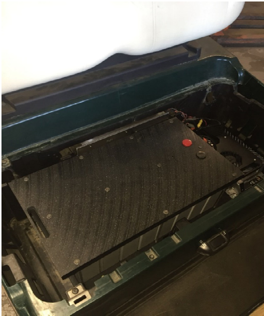
Fig. 18-Lithium battery pack installed into golf car
