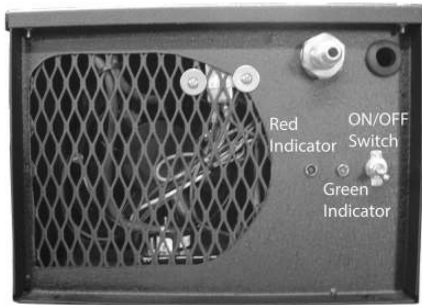
Figure 3: Side View of HC Heater (Indicator Face)
