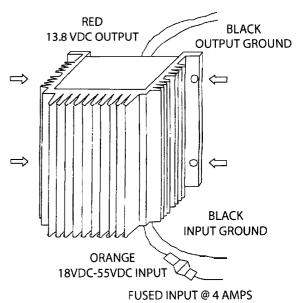
Both black wires must be connected due to the high currents developed in this unit.
