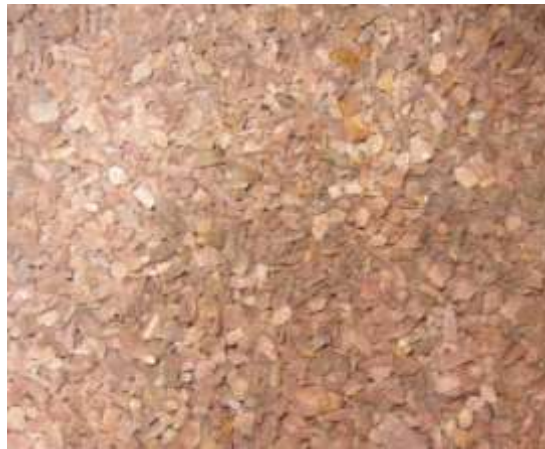
Figure 3: Example of Crushed Rock (Quartzite)
